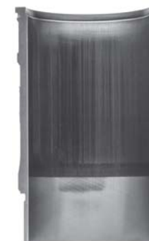
Severely Scuffed Liner
